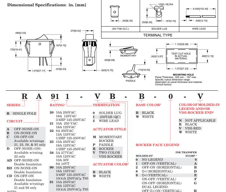
Shading indicates standard configurations.
