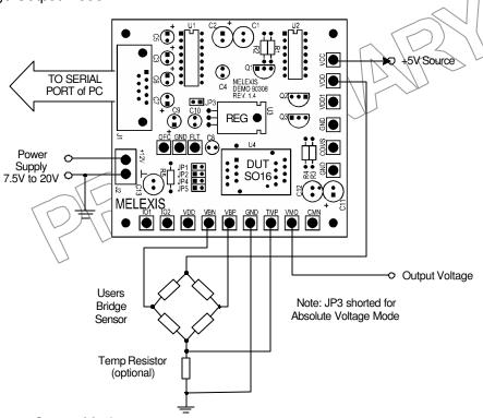
Ratiometric Voltage Output Mode:
