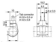
For pipe diameter (PD): ø13.5, 15, 18, 19 and 22 mm
