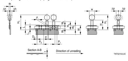
Lead spacing F = 7.5 mm (taping based on IEC 60286-2)
