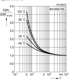
Equivalent series resistance ESR versus frequency f Typical behavior for 2200 µF/40 V
