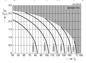
Useful life depending on case temperature  $T_C$  under ripple current operating conditions at  $V_R^{\,1)}$
