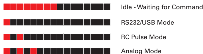
FIGURE 15. Normal Operation Flashing Patterns
