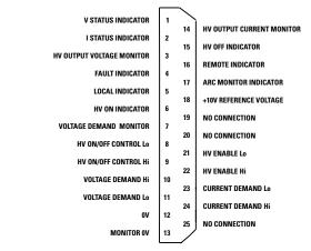
All logical indicators are open collector outputs rated at 16V (max) in the off state. An internal  $100\Omega$  resistor is connected in series with the open collector transistor. The pull down voltage is 0.9V plus the internal resistor drop.
