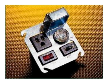
Box cover units provide an economical method of protecting small motors against overcurrent damage. For use with Edison-Base plug fuses (TOO, TLO) or Type S plug fuses (SOO, SLO) with adapters (SAO).
