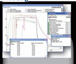
In addition to the monitor view, PicoLog can also display a graph, a spreadsheet and user notes. It can display them all at once, as shown here, or individually in any combination.
