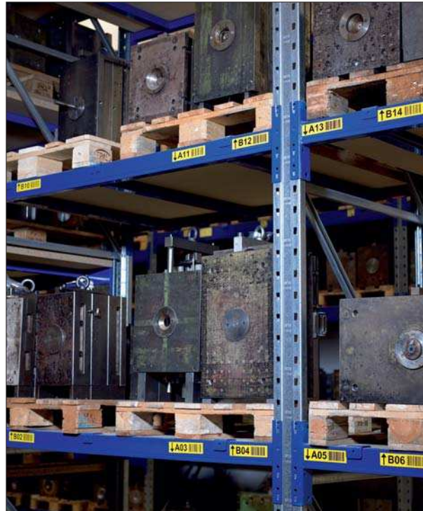
Warehouse labelling large enough to easily identify stores material.
