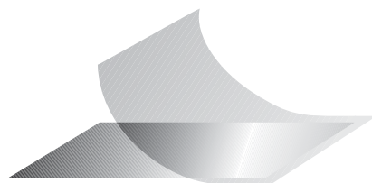
The printed silver type plate (Mat. 951A) is protected by the transparent laminate (Mat 951B).
