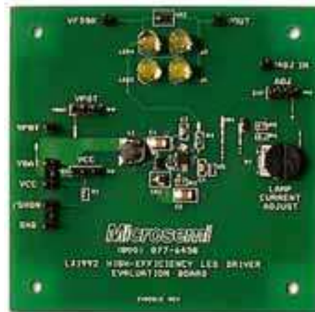
Figure 5: LX1992 Engineering Evaluation Board
