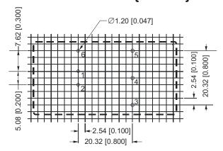
$\begin{array}{l} Pin\ section\ tolerances: \pm 0.10mm[\pm 0.004inch] \\ General\ tolerances: \pm 0.25mm[\pm 0.010inch] \end{array}$
