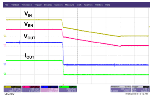
Power OFF ( R_L=8\Omega )
