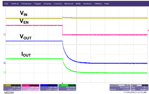
Enable OFF Sequence ( R_L=8\Omega ) VEN=2V to 0V
