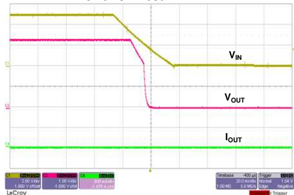
Power Off Test
