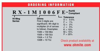
These Hi-Meg resistors are designed for use in electrometer circuits where a high order of performance is required. These resistors achieve a high degree of accuracy and stability, and operate at this high performance level for an extended period of time. By being vacuum sealed in a glass envelope, these Hi-Megs are suitable for ultra-high vacuum applications.
