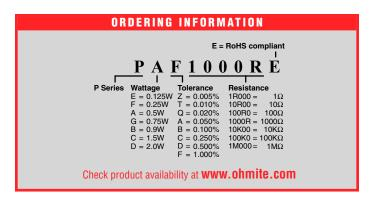
Ohmite's P Series Epoxy molded Precision Wirewound Resistors are designed to meet the exacting requirements of Military Specification MIL-R-93. The P Series offers high stability and low Temperature Coefficient of Resistance (TCR). These resistors offer tolerances as accurate as ±0.005% and Temperature Coefficients of Resistance (TCR) as low as ±2PPM/°C in a wide range of resistance values.
