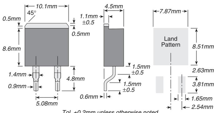
DPAK style power package for surface mounting applications; 35W power rating at 25°C case temperature.
