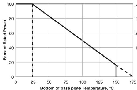
Derating (thermal resistance): 0.23W/°C (4.28°C/W). The case temperature is to be used for purposes of establishing the applied power limit. The case temperature measurement must be made with a thermocouple contacting the center of the component mounted on the designed heat sink. Thermal grease should be applied properly.
