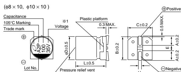
※1. Voltage mark for 6.3V is 「6V」. In case of marking for  $\phi 3$  units, "V" for rated voltage is omitted.
