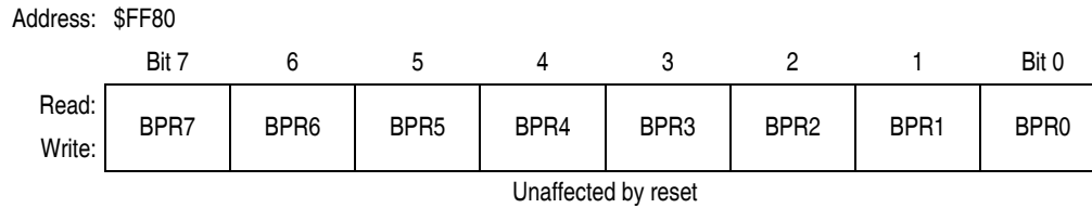
Figure 2-4. FLASH-1 Block Protect Register (FL1BPR)
