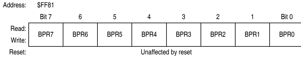
Figure 2-8. FLASH-2 Block Protect Register (FL2BPR)
