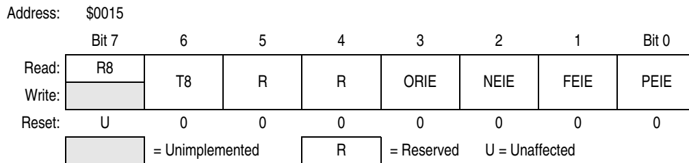
Figure 15-12. ESCI Control Register 3 (SCC3)
