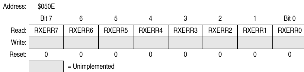
Figure 12-25. Receiver Error Counter (CRXERR)
