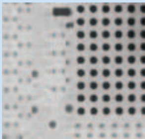
Using Teradyne's patented reconstruction techniques the overlapping capacitors can be totally removed from the image. ClearVue techniques allow for the complete dynamic range of the image to be retained, providing maximum fault coverage on this BGA and all other component types.
