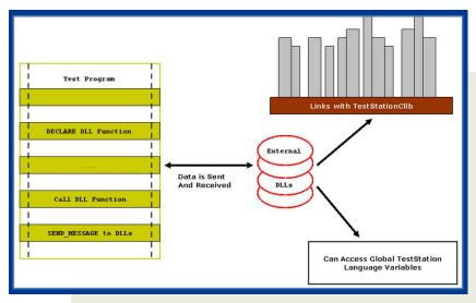
Create Dynamic Link Library application programs and link to the TestStation Runtime System.
