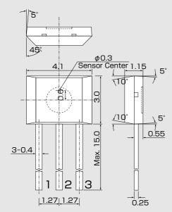
Note) The sensor center is located within the  $\phi$ 0.3mm circle.
