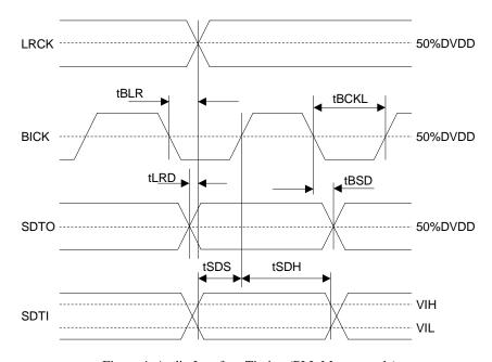
Figure 4. Audio Interface Timing (PLL Master mode)
