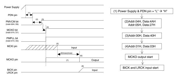
Figure 49. Clock Set Up Sequence (3)
