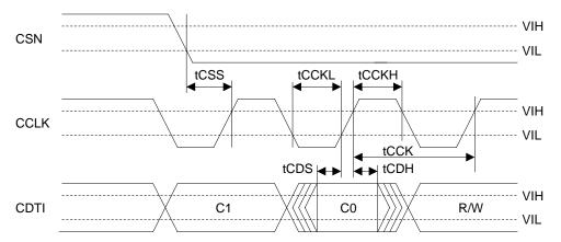
Figure 8. WRITE Command Input Timing
