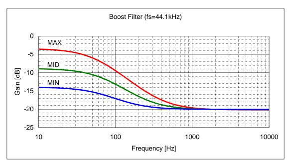
Figure 27. Bass Boost Frequency Response (fs=44.1kHz)
