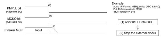
Figure 56. Clock Stopping Sequence (3)
