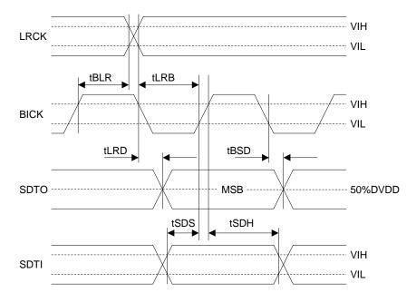
Figure 7. Audio Interface Timing (PLL/EXT Slave mode)
