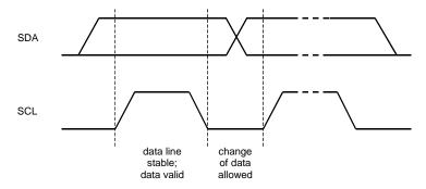
Figure 44. Bit Transfer on the I<sup>2</sup>C-Bus
