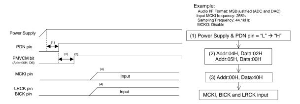
Figure 50. Clock Set Up Sequence (4)
