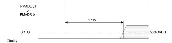
Figure 11. Power Down & Reset Timing 1
