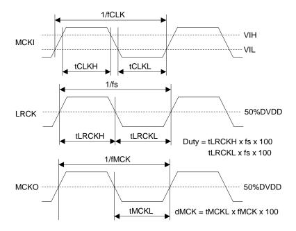
Figure 3. Clock Timing (PLL Master mode)
