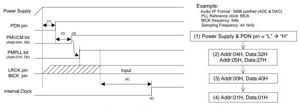
Figure 48. Clock Set Up Sequence (2)
