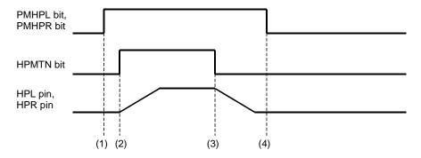
Figure 33. Power-up/Power-down Timing for Headphone-Amp
