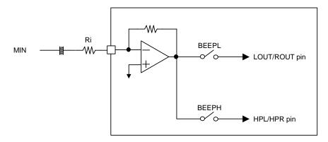
Figure 29. Block Diagram of MIN pin
