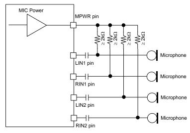
Figure 23. MIC Block Circuit
