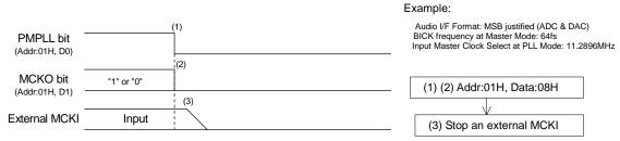
Figure 54. Clock Stopping Sequence (1)
