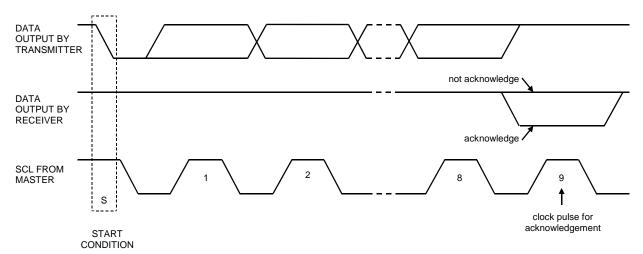
Figure 43. Acknowledge on the I<sup>2</sup>C-Bus
