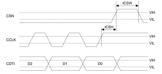
Figure 9. WRITE Data Input Timing
