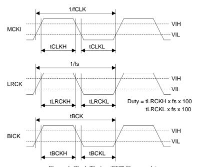
Figure 6. Clock Timing (EXT Slave mode)
