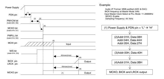
Figure 47. Clock Set Up Sequence (1)
