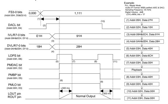
Figure 53. Stereo Lineout Sequence
