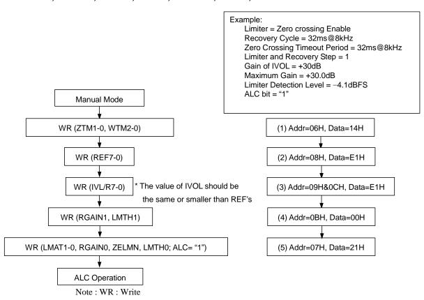
Figure 25. Registers set-up sequence at ALC operation
