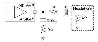
Figure 34. External Circuit Example of Headphone
