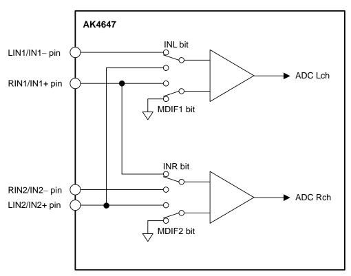
Figure 21. Mic/Line Input Selector
