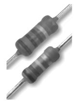
A homogenous film of metal alloy is deposited on a high grade ceramic body. After a helical groove has been cut in the resistive layer, tinned electrolytic copper wires are welded to the end-caps. The resistors are coated with a blue, non-flammable lacquer, which provides electrical, mechanical, and climatic protection.
