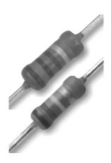
A homogenous film of metal alloy is deposited on a high grade ceramic body. After a helical groove has been cut in the resistive layer, tinned electrolytic copper wires are welded to the end-caps. The resistors are coated with a blue, non-flammable lacquer, which provides electrical, mechanical, and climatic protection.
