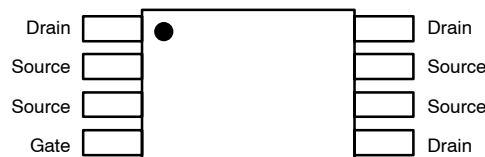
Figure 2. Pinouts for Single Die TSSOP
