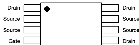
Figure 2. Pinouts for Single Die TSSOP
