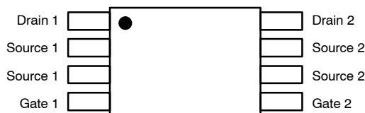
Figure 3. Pinouts for Dual-Die TSSOP
