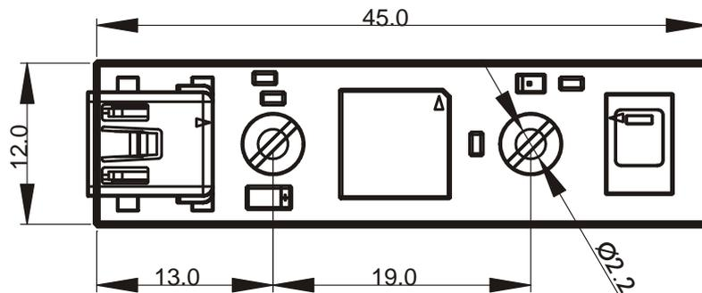
Figure 1: Mechanical dimensions of the Oak RH sensor
