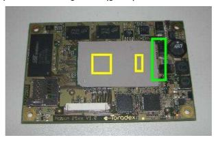
4. On attaching the heatsink, make sure the yellow marked corner is on the right side. (Very important for Robin since she position of the screws don't assure that it is mounted correctly).
