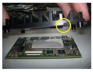
5. Mount the heatsink in a way that the position of the holes is right from the beginning (moving it may not be possible since the TIM sticks the aluminium and print together).
