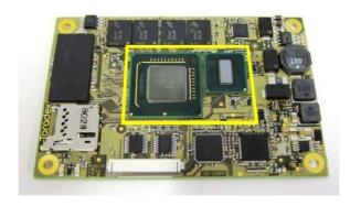
2. Remove the plastic foils on the TIM (on both sides) and attach the TIM as shown over the SCH and CPU.
