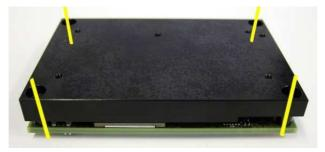
6. Use M2.5 screws to fix the heatsink together with module.
