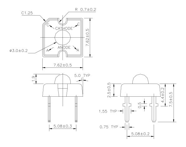
Note: 1. Tolerances unless mentioned  $\pm 0.25$ mm. Unit = mm
