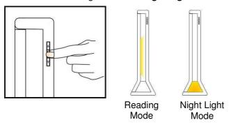
4. When it is in **Reading Mode**, clicking up and down arrow buttons can adjust brightness. Step dimming function:
