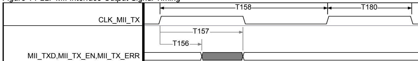
Figure 14-22. MII Interface Output Signal Timing
