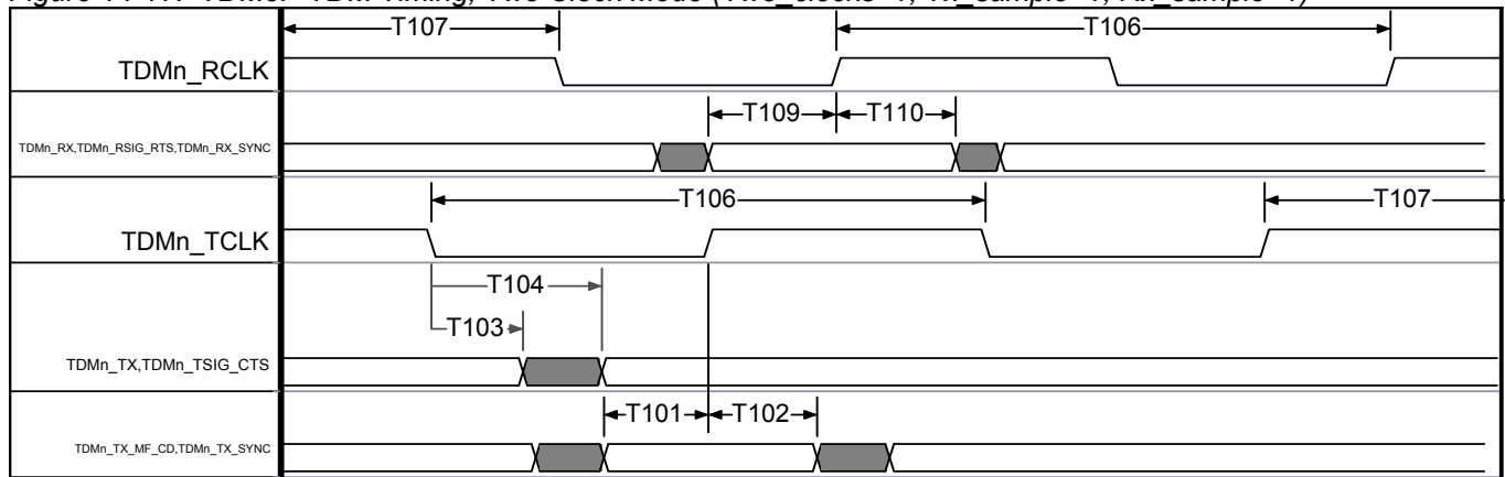
Figure 14-17. TDMoP TDM Timing, Two Clock Mode (Two_clocks=1, Tx_sample=1, Rx_sample=1)
