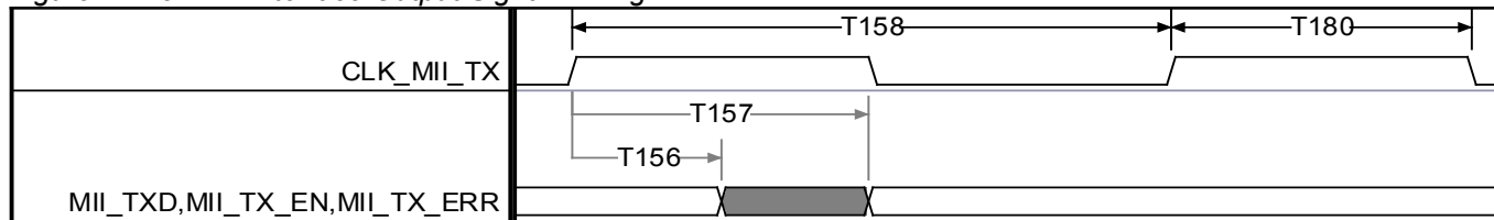
Figure 14-15. MII Interface Output Signal Timing
