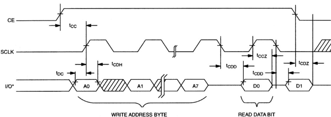
**TIMING DIAGRAM: 3-WIRE WRITE DATA TRANSFER** Figure 10
