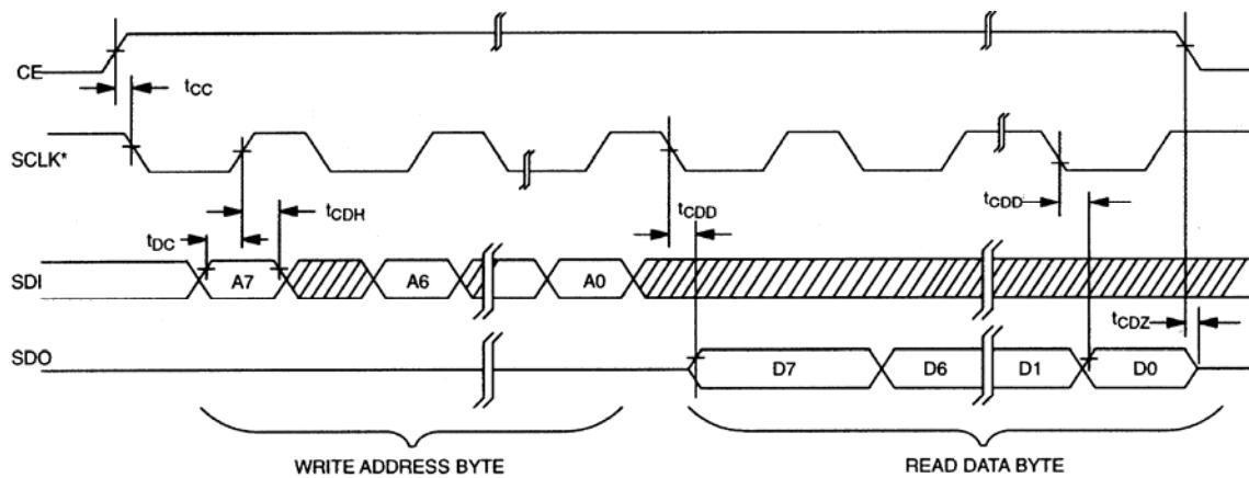
**TIMING DIAGRAM: SPI WRITE DATA TRANSFER** Figure 12
