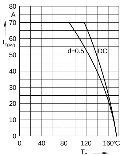
Fig. 4 Average forward current I_{F(AV)} versus case temperature T_C
