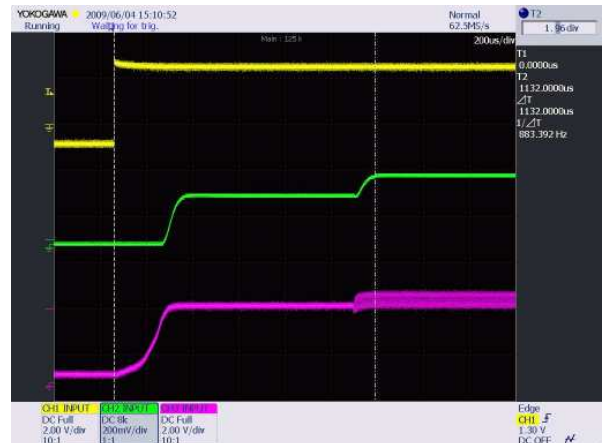
V_{IN} = 3.6\text{ V} , Ch1 – PWM, Ch2 – LED current (200 mA/div), Ch3 – Output voltage
