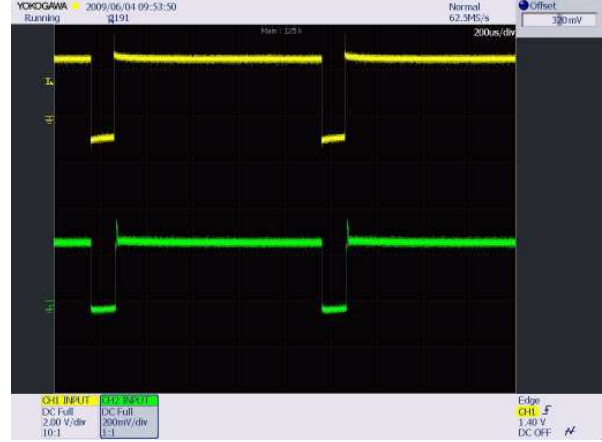
V_{IN} = 4.2\text{ V} , Ch1 – PWM, Ch2 – LED current (200 mA/div)
