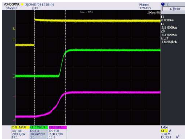
V_{IN} = 4.2\text{ V} , Ch1 – PWM, Ch2 – LED current (200 mA/div), Ch3 – Output voltage
