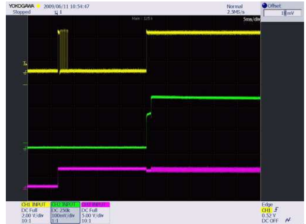
V_{IN} = 3.6\text{ V} , Ch1 – EN/SET, Ch2 – LED current (200 mA/div), Ch3 – Output voltage
