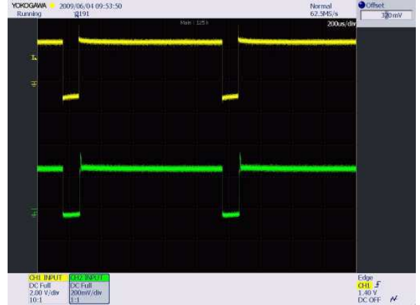
V_{IN} = 4.2\text{ V} , Ch1 – EN/SET, Ch2 – LED current (200 mA/div)
