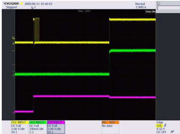
V_{IN} = 4.2\text{ V} , Ch1 – EN/SET, Ch2 – LED current (200 mA/div), Ch3 – Output voltage
