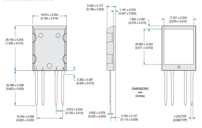
NOTE: Back-side heat sink meets  $2500V_{\rm rms}$  isolation to the pins.
