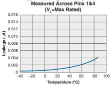
Typical Leakage vs. Temperature
