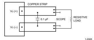
Note: Use a 0.1 µF ceramic capacitor. Scope measurement should be made using a BNC socket. Position the load between 50.8 mm and 76.2 mm (2 in. and 3 in.) from the module.
