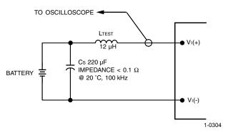
Note: Input reflected-ripple current is measured with a simulated source impedance of 12  $\mu$ H. Capacitor Cs offsets possible battery impedance. Current is measured at the input of the module.
