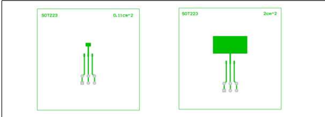
Figure 19. SOT-223 PC board (1)
