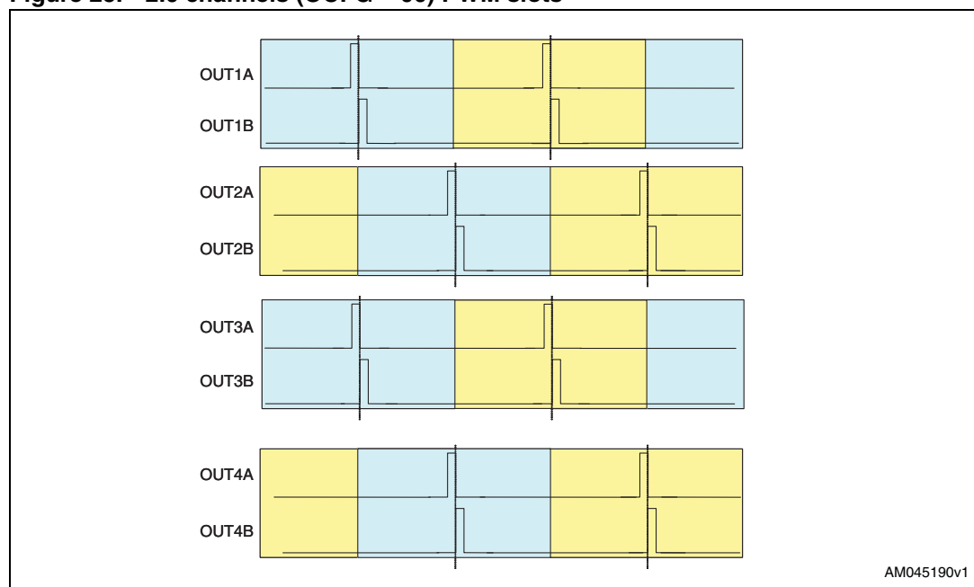
Figure 25. 2.0 channels (OCFG = 00) PWM slots
