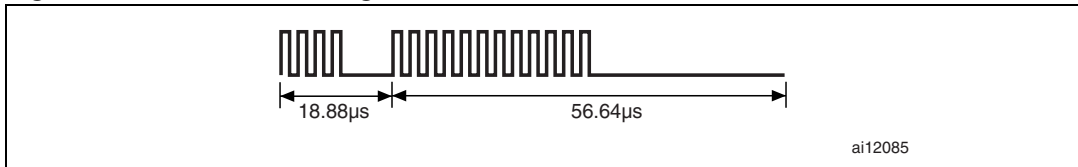
Figure 30. End of frame, high data rate, one subcarrier x2
