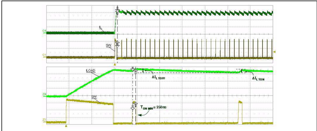
Figure 20. Short-circuit current V_{IN} = 24\text{ V}
