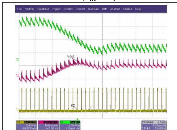
Figure 47. Zoom - 1 A to 3 A falling edge load transient ( V_{IN} 32 V)
