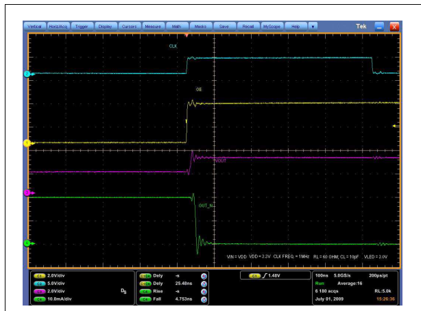
Figure 16. Turn ON output current characteristics (1)
