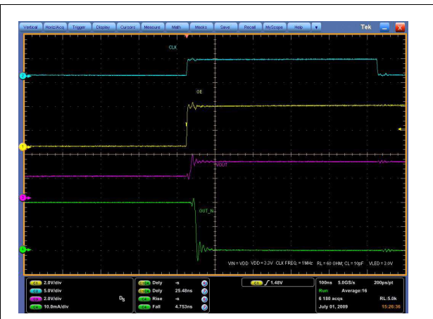
Figure 17. Turn OFF output current characteristics (2)
